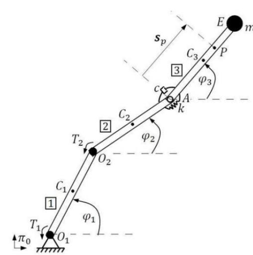
Figure: Manipulator with three degrees of freedom
