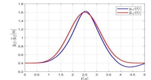
Figure: Comparison of desired and simulated output trajectories for 3DOF manipulator.
