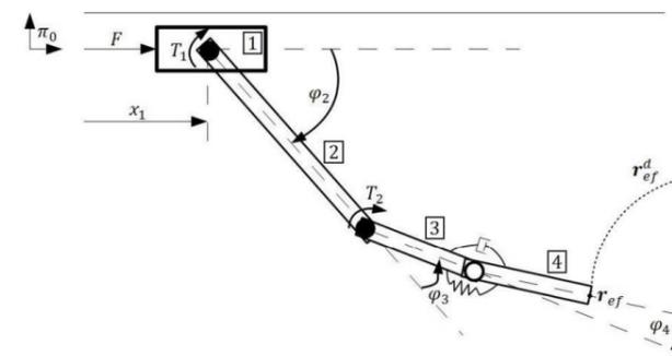
Figure: Manipulator with four degrees of freedom.
