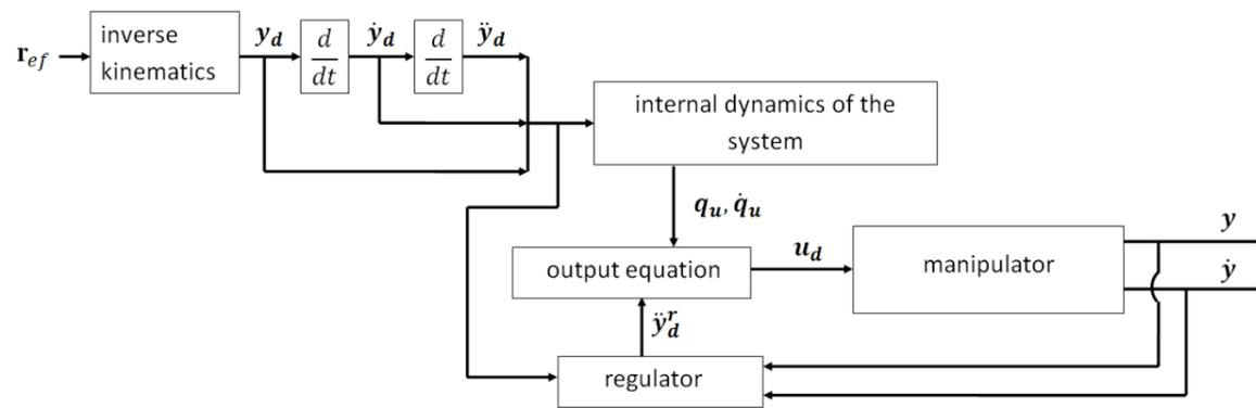
Figure: Schema of control system for underactuated manipulator obtained with method of linearly combined output.
