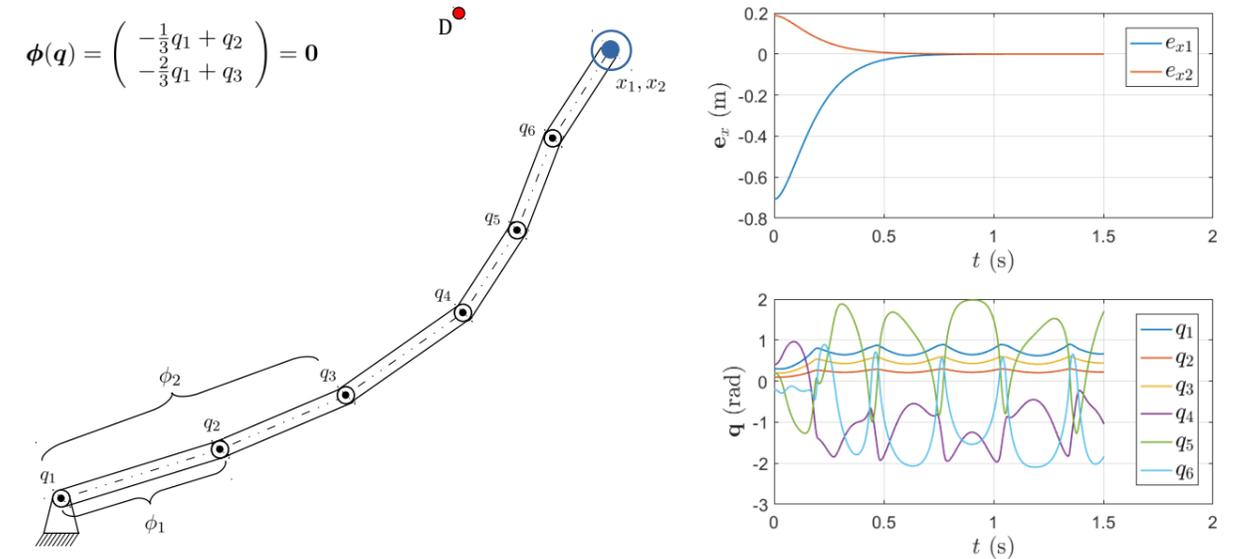
**Figure:** Operational space control of 6-DOF planar manipulator with two kinematic couplings  $\phi_1, \phi_2$  and destination point  $D$ . The quantity  $e_x = \mathbf{x}_d - \mathbf{x}$  is the position control error in time  $t$  and  $\mathbf{q}$  is the vector of generalized position variables.  $\boldsymbol{\tau}_o = -k_N \nabla U$  is chosen to minimize the gravity effort, defined as  $U = \|\mathbf{G}(\mathbf{q})\|^2$ .
