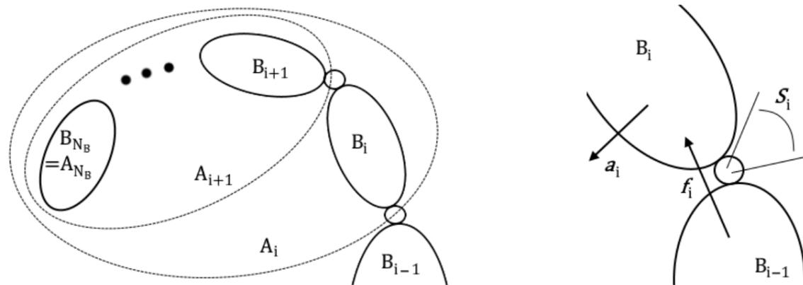
**Figure:** Primary aspects of the *articulated-body* algorithm: (Left) the way of defining the articulated bodies  $A_i$ , (Right) the idea of searching for acceleration  $\ddot{q}_i$  corresponding to joint  $i$ .  $N_B$  is the number of rigid bodies.
