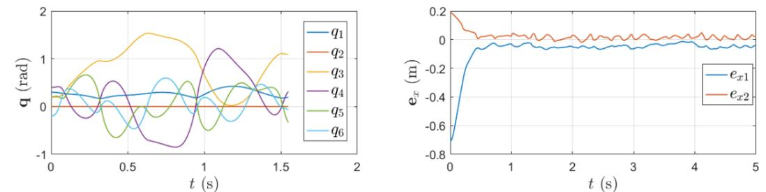
**Figure:** Two interesting cases of control of 6-DOF planar manipulator: (Left) with the only constraint equation  $q_2 = 0$  and  $\boldsymbol{\tau}_o = \mathbf{0}$ , (Right) having assumed  $\phi_1, \phi_2, \boldsymbol{\tau}_o = -k_N \nabla U$  and 20% uncertainty in mass of bodies.
