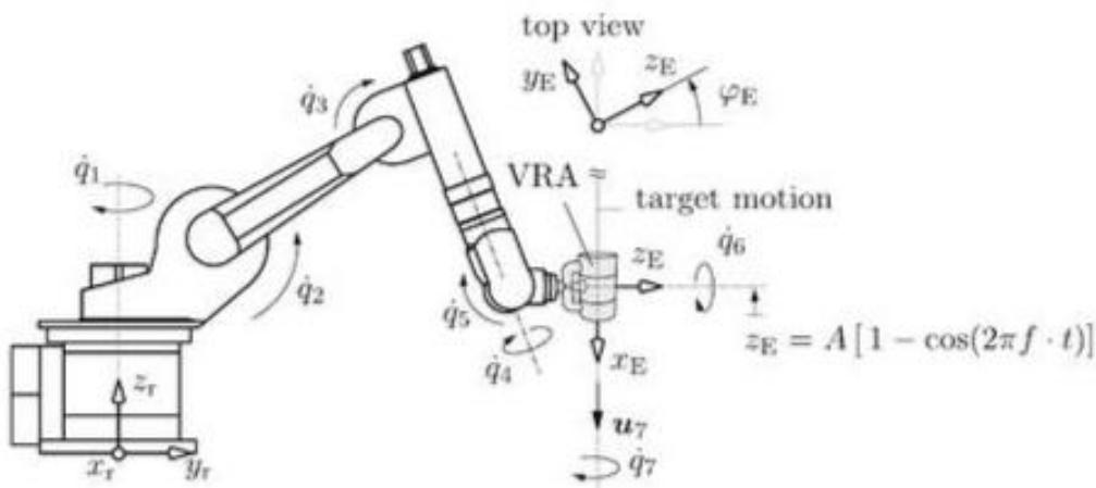
**Figure:** Vertical motion with constant orientations. F. Geu Flores, S. Rottgermann, B. Weber, A. Kecskemethy: Robust Inverse Kinematics at Position Level by Means of the Virtual Redundant
