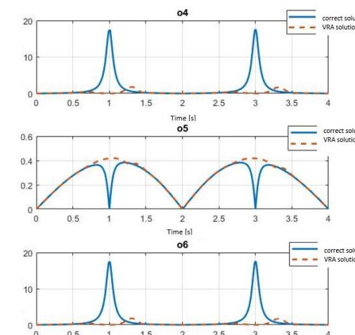
Figure 1 Joint velocities [rad/s] in the wrist
