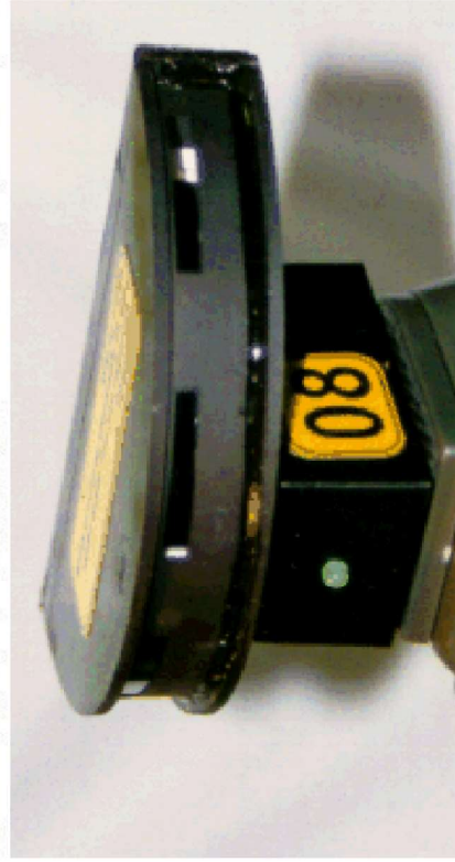
Figure 6.21: The C omputerized O pto-electronic N avigation and C ontrol (CONAC TM ) system employs an onboard, rapidly rotating and vertically spread laser beam, which sequentially contacts the networked detectors. (Courtesy of MTI Research, Inc.)
