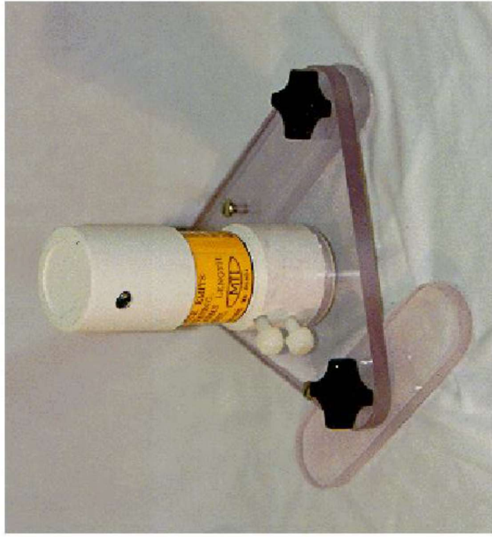
Figure 6.21: The C omputerized O pto-electronic N avigation and C ontrol (CONAC TM ) system employs an onboard, rapidly rotating and vertically spread laser beam, which sequentially contacts the networked detectors. (Courtesy of MTI Research, Inc.)
