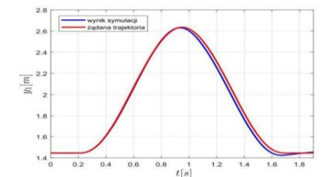
Figure: Comparison of desired and simulated output trajectories for 4DOF manipulator.
