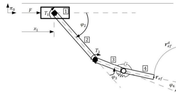
Figure: Manipulator with four degrees of freedom.
