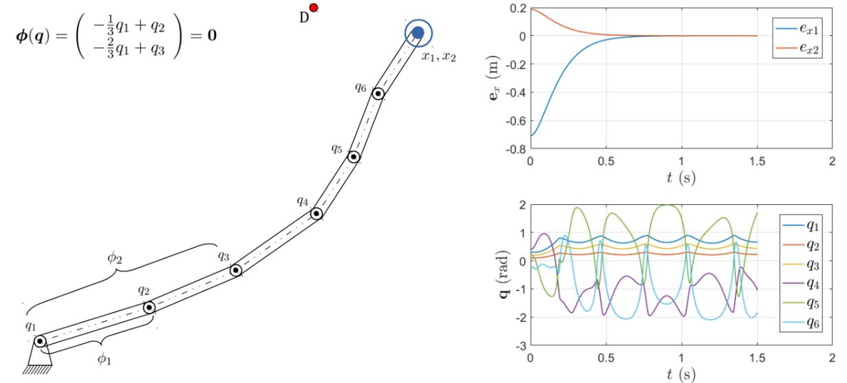
**Figure:** Operational space control of 6-DOF planar manipulator with two kinematic couplings  $\phi_1, \phi_2$  and destination point  $D$ . The quantity  $e_x = x_d - x$  is the position control error in time  $t$  and  $q$  is the vector of generalized position variables.  $\tau_o = -k_N \nabla U$  is chosen to minimize the gravity effort, defined as  $U = \|G(q)\|^2$ .
