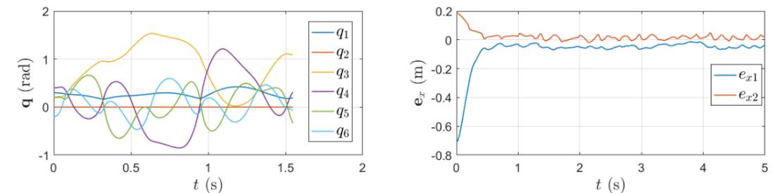
**Figure:** Two interesting cases of control of 6-DOF planar manipulator: (Left) with the only constraint equation  $q_2 = 0$  and  $\tau_o = 0$ , (Right) having assumed  $\phi_1, \phi_2, \tau_o = -k_N \nabla U$  and 20% uncertainty in mass of bodies.
