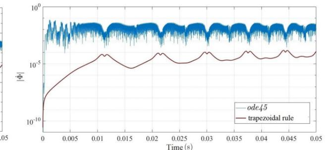
Figure: Constraint violation for velocities  $\dot{\mathbf{q}}$
