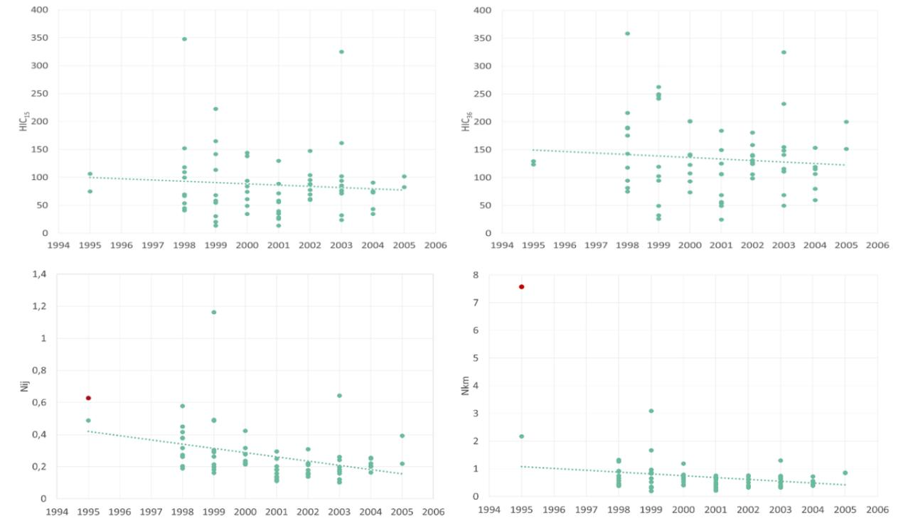
**Figure:** Injury criteria values (HIC15, HIC36, Nij, Nkm) for the dummy on the driver's seat in rear collisions
